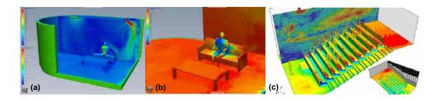
**Figure 5** Example of PMV value and velocity slice place (a) and PPD result (b) of thermal comfort simulation result: (Autodesk Simulation CFD 2013) and Example of surface irradiation (c) of main lecture room: (STAR-CCM+ Building services 2013)
