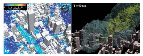
**Figure 4** Example of wind pattern between buildings of Manhattan (a) and at 9/11 building collapse smoke (b):(Alan Huber 2006)
