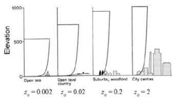
Figure 1 Mean wind profiles for different terrains: (P. Mendis 2007)
