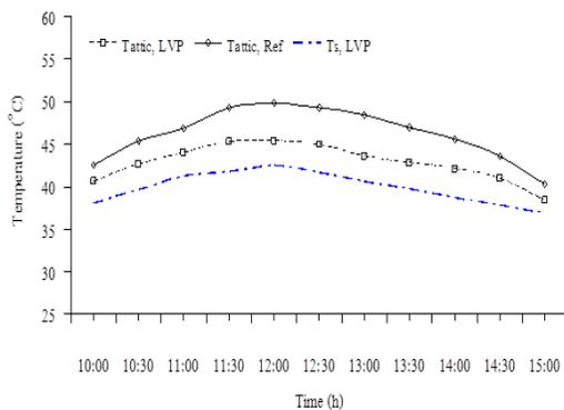
**Fig. 4.** Attic temperature and LVP surface temperature.
