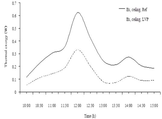
**Fig. 16.** Hourly variation of exergy ceiling heat gain.
