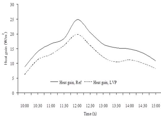
**Fig. 15.** Hourly variation of ceiling heat gain.
