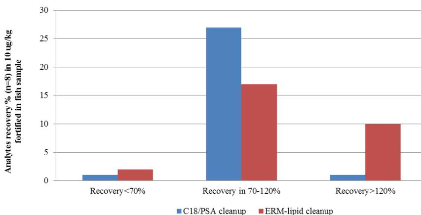
**Fig. 4.** Number of analytes with % recoveries within the acceptable % recovery range 70-120% for C18/PSA cleanup and ERM-lipid cleanup at 10  $\mu\text{g}/\text{kg}$ .
