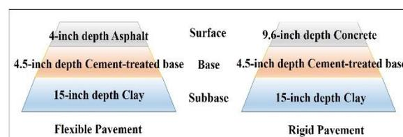
**Figure 2** Design structures used in the hypothetical case study
