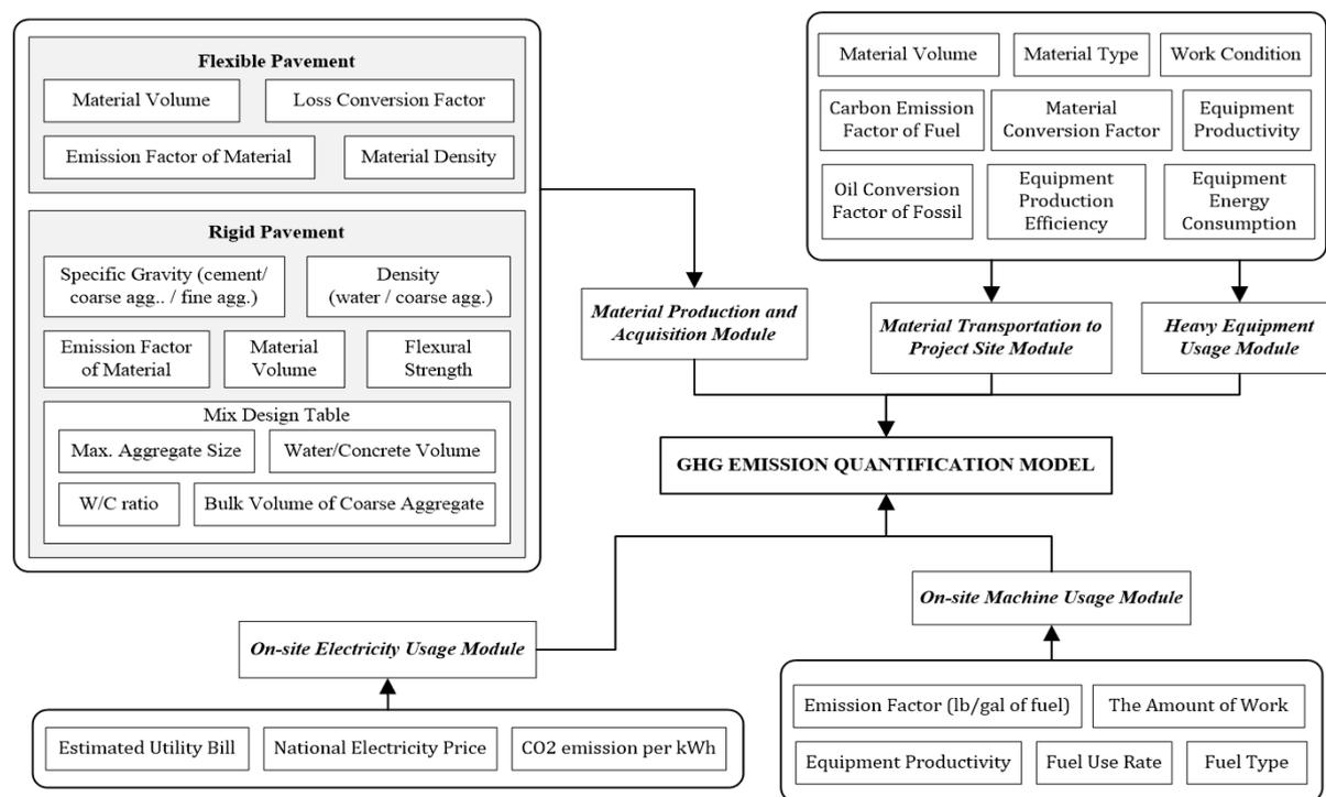
**Figure 1** Schematic framework of the GHG emission quantification model
