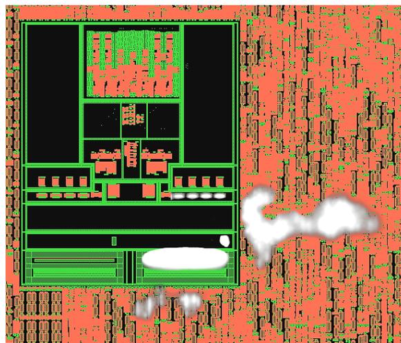
**Figure 6** Latchup propagation in a semiconductor chip
