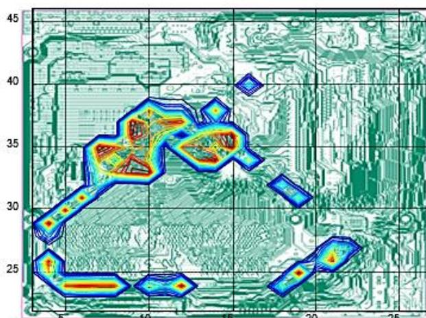
**Figure 8** ESD-EMC scan of a printed circuit board (PCB) highlighting sensitivity to electromagnetic interference (EMI)
