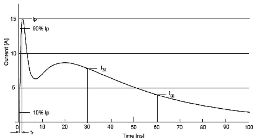
**Figure 5** IEC 61000-4-2 pulse waveform
