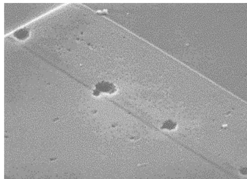
**Figure 2** Charged device model (CDM) failure in a MOSFET gate region
