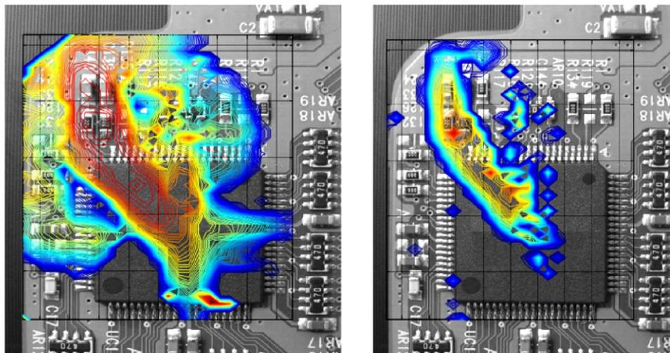
**Figure 7** ESD-EMC sensitivity of scanning method comparison of two products
