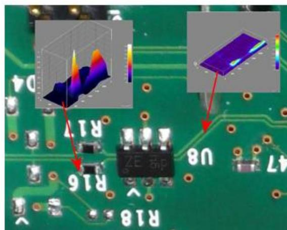
**Figure 9** Current reconstruction electromagnetic signal scanning technique
