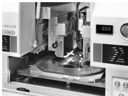
**Figure 3** Commercial wafer level ESD test system
