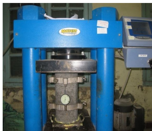
Figure 7 Test on Modulus of Elasticity of HSHFC
