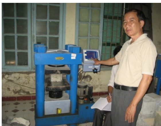
Figure 6 Compression Test on HSHFC on the Compression Machine Mates 3000KN - Italy
