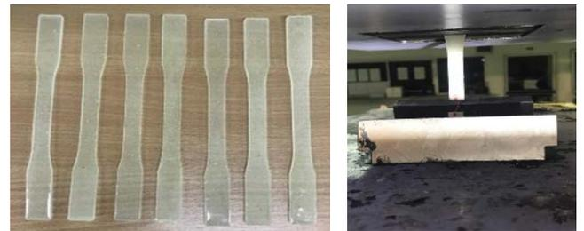
**b)** Epoxy resin and test setup
