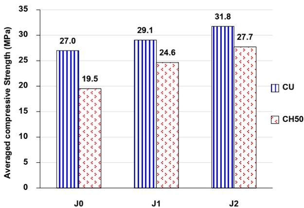
Figure 8 Effect of JNFRP's layers on compressive strength of concrete cylinders subjected to a room temperature and 50 °C
