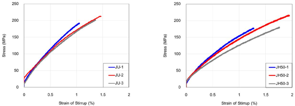
Figure 4 Stress-strain relationships of JNFRP coupons subjected to a room temperature and 50 °C
