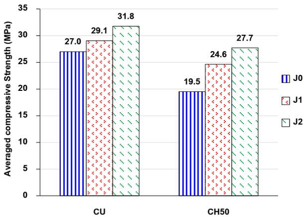
Figure 7 Effect of temperature on compressive strength of concrete cylinders subjected to a room temperature and 50 °C
