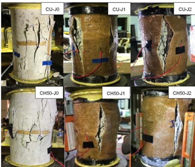
Figure 6 Failure modes of unconfined and confined concrete cylinders
