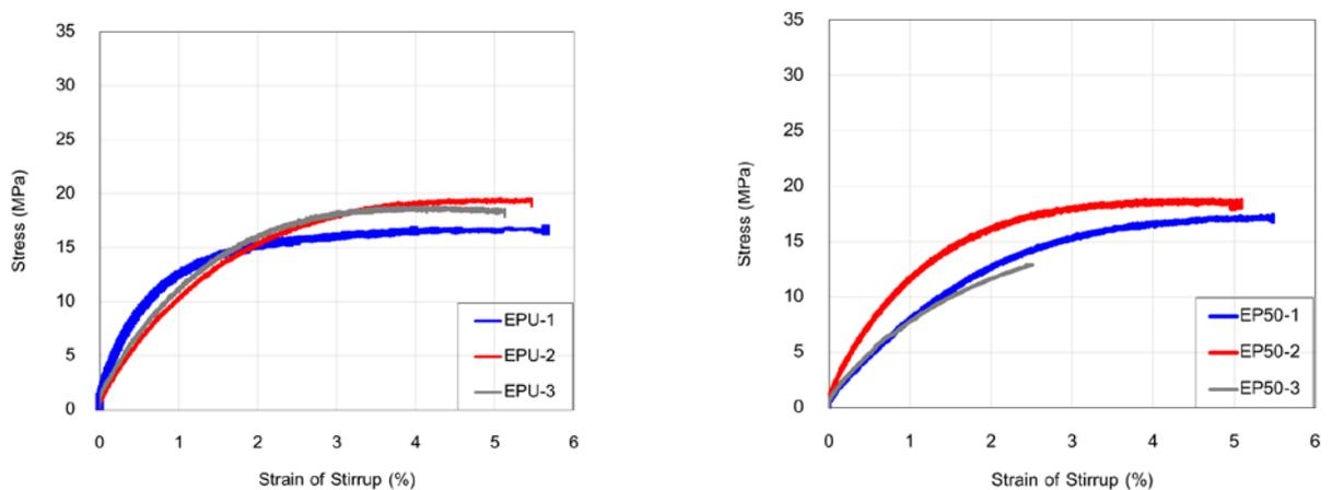
Figure 5 Stress-strain relationships of epoxy-resin coupons subjected to a room temperature and 50 °C
