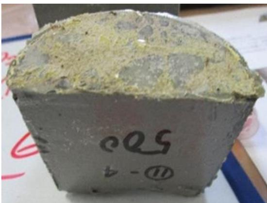
**Figure 8** Specimen coating with gel.
