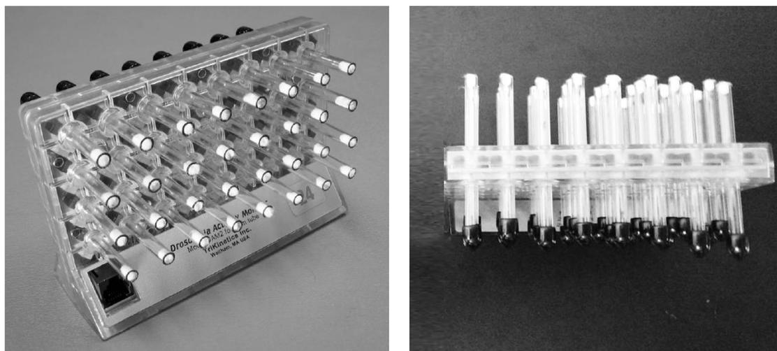
**Figure 3** Infrared beam-split movement monitors [11]
