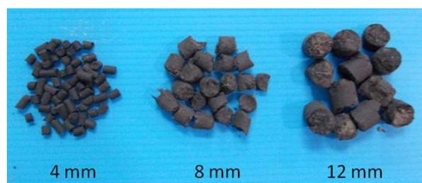
Figure 3 The aggregate sample of growing media from filter cake and bagasse ash
