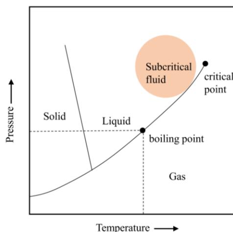
**Figure 3** Schematic phase diagram of substance showing subcritical fluid area.
