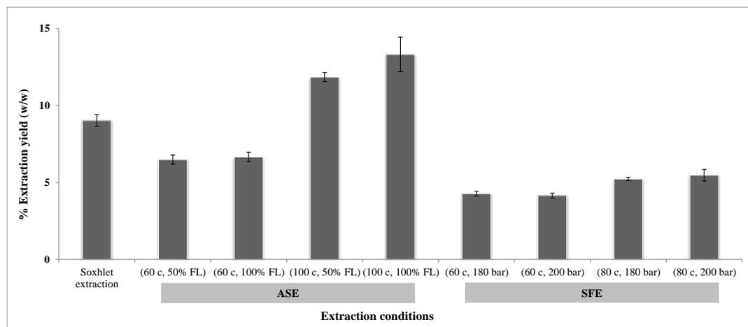
**Figure 1** Crude wax extraction yield (w/w dried sugarcane filter cake) obtained from Soxhlet extraction, four condition of ASE (60 °C and 100 °C extraction temperature and 50% and 100% flushing volume (FL)) and four conditions of SFE (60 °C and 80 °C extraction temperature and 180 and 200 bar).
